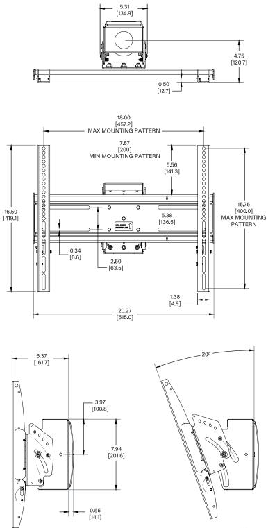
Measurements within brackets [xx.xx] are mm, measurements outside of brackets are inches.
